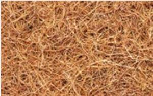
**Coconut, jute, or other organic fiber grids:** They control erosion in furrows and gullies on slopes, helping germination and root formation. They are commonly adjusted with live stakes or plant establishment systems to establish long term live barriers. Their high resistance allows them to be used in some cases to replace rockfills. The coconut fiber rolls can be mixed with other products or erosion control systems.
