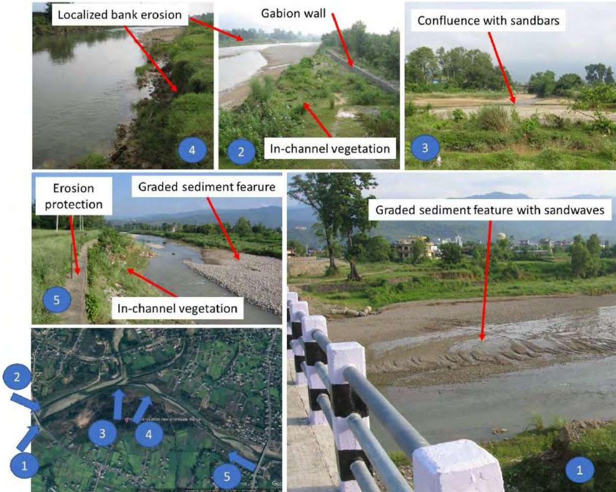
Figure 2-3 A pictorial impression associated with sediment, morphology and vegetation features in the reach at the project site
