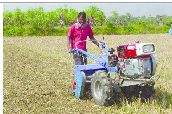
Soil cultivation and sowing in one pass with a mechanical seed drill (Photo : E.M. Haque, CIMMYT Bangladesh)
