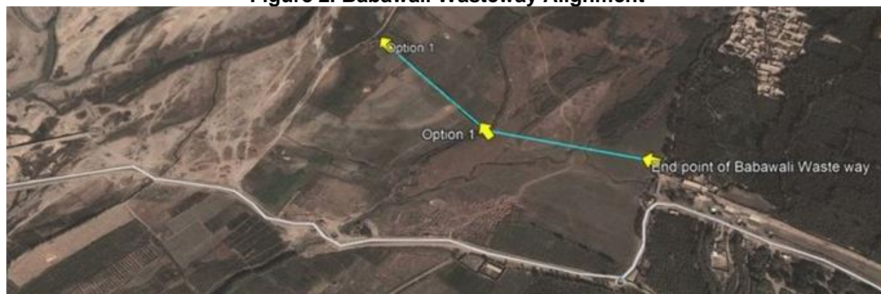
Figure 2. Babawali Wasteway Alignment
