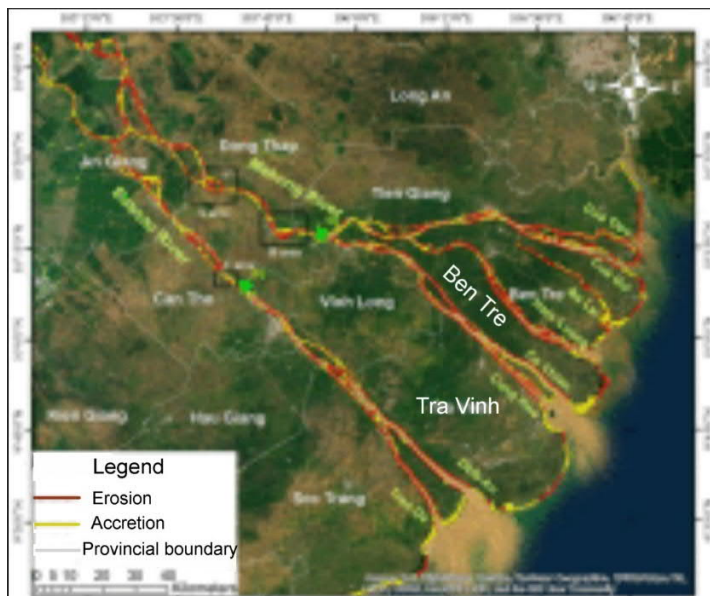
Figure 37. Erosion and accretion along the major rivers through the project area (1989-2014)
